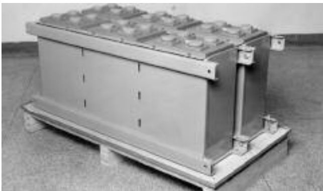
Figure 2: The modules bolted together and to the pallet using transit bolts
