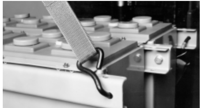
Figure 3: Lifting strap/hook attached to a module
